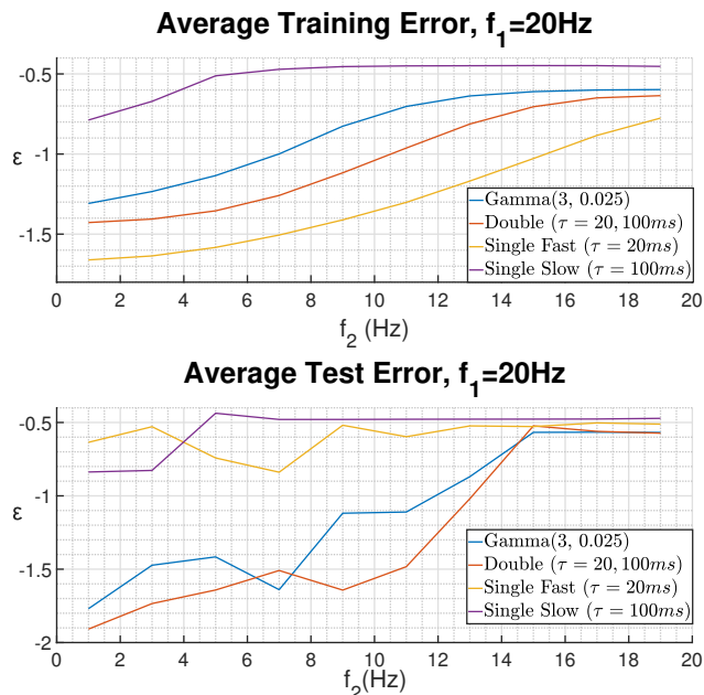
Figure 1: Training and test error averaged over 10 trials for a 1000 LIF network trained using the FORCE method to reproduce a sum of two sinusoids signal at frequencies f_1 = 20\text{Hz} and f_2 . Synapses were either all fast or all slow (Single Fast, Single Slow), split randomly into a fast and slow group (Double), or fully randomly distributed (Gamma).
